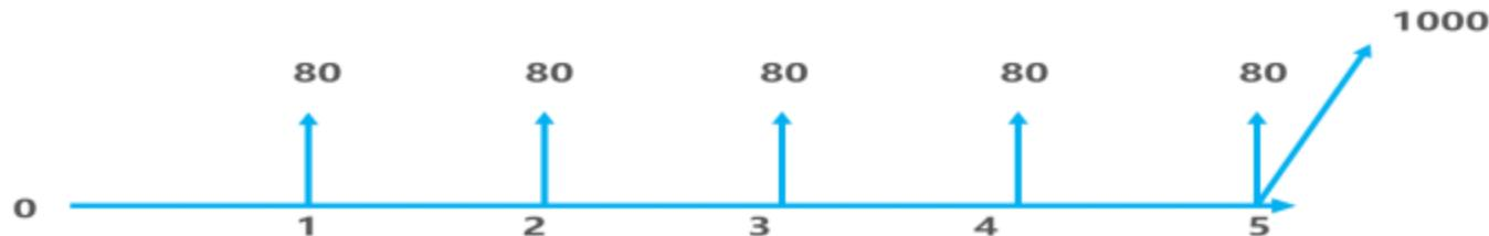
$$\begin{aligned} PV &= 80 \times (P/A, 10\%, 5) + 1000 \times (P/F, 10\%, 5) \\ &= 80 \times 3.791 + 1000 \times 0.621 \\ &= 924.28 \text{ (元)} \end{aligned}$$
